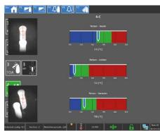
Uniquely the XPAR Vision GobAssist-BTC is integrated with major IS-machine timing systems to enable closed loop interfaces for automatic Mould Cooling and Glass Distribution control.
