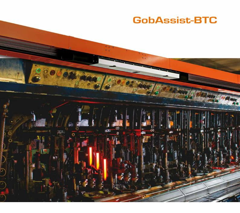
Hot End sensor solution for monitoring and controlling of gob loading and temperature of the blank mould, neck ring, plunger and parison
