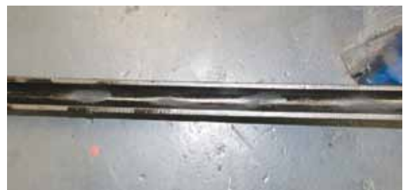
Figure 4: Worn out deflector.
