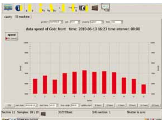
Figure 5: Gob speed differences between sections.
