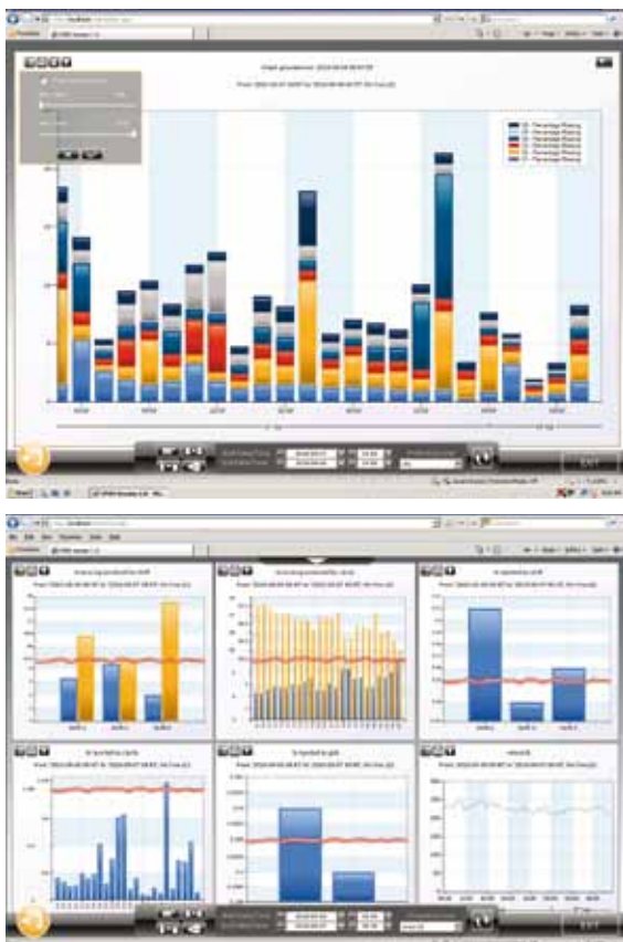
Figure 8: XPAR Vision's XMIS system; shown here are a typical graph and dashboard with hot end process data.
