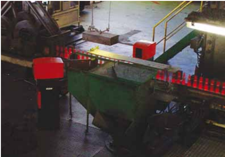
Figure 2: XPAR Vision hot end infrared camera system for inspection and process monitoring and control.
