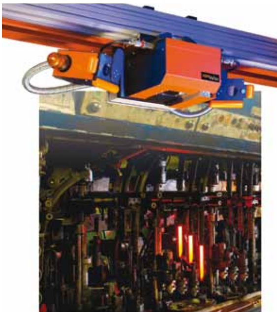
Figure 7: The BTC is an add-on to the Gob Assist and glides along the same rail system.
