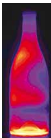
Figure 2: With two cameras positioned at an angle on each side of the conveyor belt directly after the forming machine, a thermal image is made of each passing bottle.
