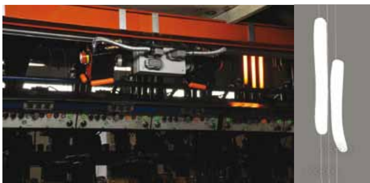
Figure 5: With the Gob Assist, images of the gob are made from the moment it leaves the deflector until the moment it has fallen completely into the blank mould.
