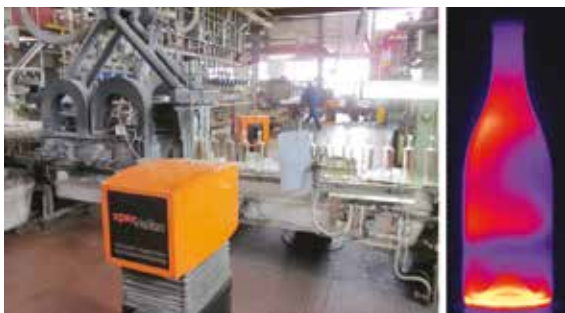
Figure 3: With two cameras positioned at an angle on each side of the conveyor belt directly after the forming machine, a thermal images is made of each passing bottle.
